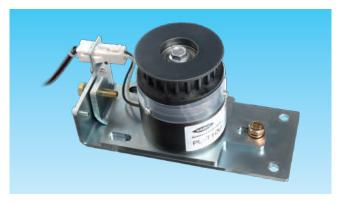
The PL-type electric lock is a device that keeps the door closed by restraining the driving belt firmly coupled to the door with the electromagnetic lock built into the idler pulley.
