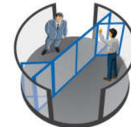
Two-wing automatic revolving doors ← The door wings of two-wing doors are fixed to the H-girder which can drive the door wings.
