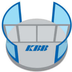
↑ KBB drum wall load-bearing
