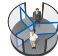
Three/Four-wing revolving doors ← The door wings of the three/four wings revolving doors are fixed to the central axis which can drive the door wings.
