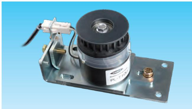
The PL-type electric lock is a device that keeps the door closed by restraining the driving belt firmly coupled to the door with the electromagnetic lock built into the idler pulley.
